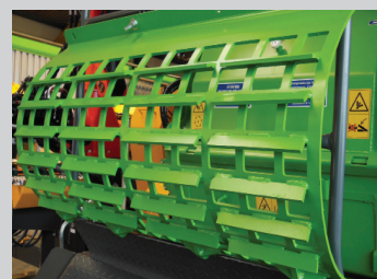
Grilles de calibrage : 25/25mm, 35/40mm, 45/60mm, 60/80mm
